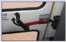
To open the emergency exit, a person must unlatch the door by pulling the red lever upward, and then push against the door. The rear emergency exit also has a separate 'vandal lock,' shown below:"
